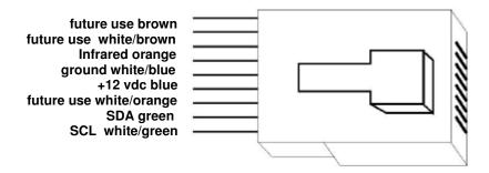
Run CAT5 wire from the keypad location to the GSZ44 location for each keypad. It isn't a bad idea to run a second cat5 wire run to each location to leave the installation more "future proof" and reliable. Leave an extra 1 m or 3 feet on each side to make it easier to work on. Add a RJ45 connector of the right type for the CAT5 wire you have selected (not all CAT5 wires are the same) and crimp the connector to the wire on each side. Plug the RJ45's into the MR40 and correct GSZ44 ports.
